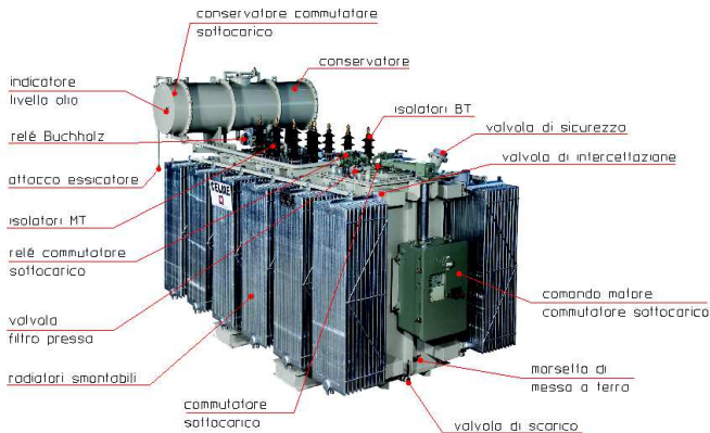
Figure 1.0.2: breathing type transformer with on load tap changer
