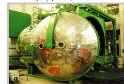
德国技术全自动真空浇注灌 Full automatic numerical steam vacuum gating systems from German
