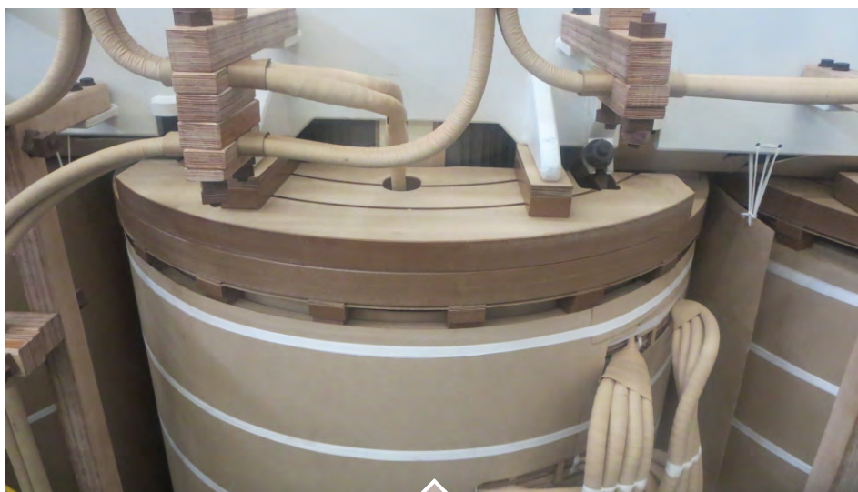
The end of the coil is the active part of special transformer with a magnetic shielding structure, which adopts a pressing process of hydraulic press with active part press.
