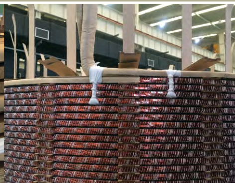
h The coil is ready to be put into oven for drying treatment
