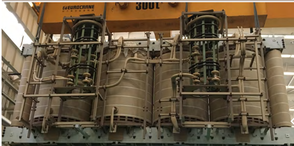
The end of the coil is the active part of special transformer with a magnetic shielding structure, which adopts a pressing process of hydraulic press with active part press.
