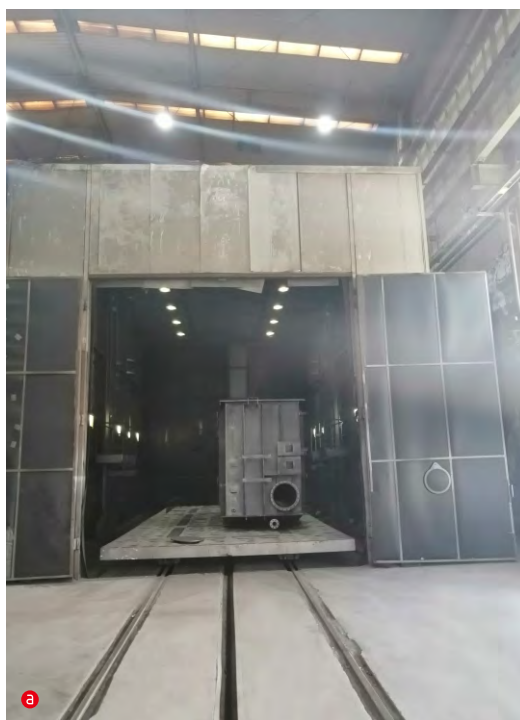
d 16m water-revolving spray booth
